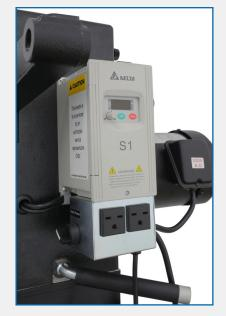
Power Inverter converts standard 240 V Electric Supply to 415 V for the 3 phase motor.
