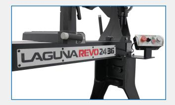
Highly Polished Steel Bed - Tool Rest glides into position, locked with the soft grip cam lever.
