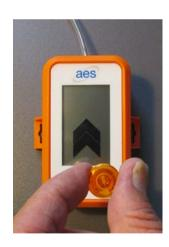
Hold a magnet to the right of the LED hole, approximately below the 'r' in 'airflow indicator' until the LED illuminates continuously. When this happens, move the magnet away from the unit and wait until the LED starts to flash. Once more, hold the magnet in the above position until the LED illuminates continuously. Now take the magnet away again.
