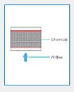
Filters small particles @ 99.997% down to 0.3 microns in size.
