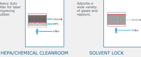
Adsorbs gases and vapours generated by ink jet printing and certain solvent applications.
