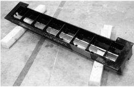
Bed with headstock and tailstock removed
