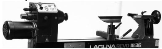
**5.** Lower the bed of the lathe onto 2 stacks of wood. This will allow access to the underside of the bed.
