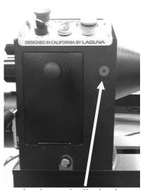
Lathe spindle lock
