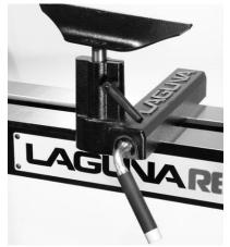
Tool rest assembled to the bed
