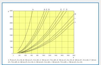
For exhaust extraction systems in vehicle repair shops where engines are running without load and with low rpm's, the following air flows can be used as guidelines:
