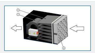
The function of the machinery is that the airborne particulate is drawn by the fan (pos. 1) into the air cleaner and through the filters (pos. 2) located at the front of the unit. The cleaned air is discharged at the rear of the unit via a double deflection grill (pos. 3).
