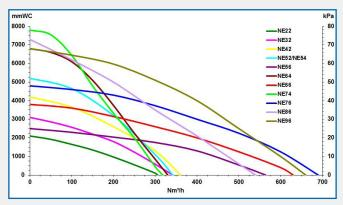
Air powered ejectors All performance data are based on 7 bar supply pressure
