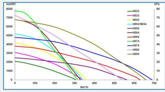
Air powered ejectors Air performance data are based on 7 bar supply pressure
