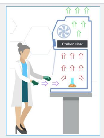
Clean Air Contaminated Air Working Environment Air
