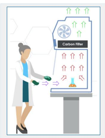
Clean Air Contaminated Air Working Environment Air
