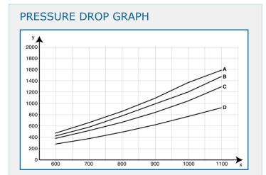
X: airflow m<sup>3</sup>/h Y: static pressure Pa A = 4 m horizontal B = 4 m vertical C = 3 m, D = 2 m
