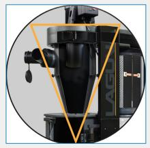
The Golden Triangle: Cyclones are designed to put the maximum amount of dust directly into the drum, without passing the fan.
