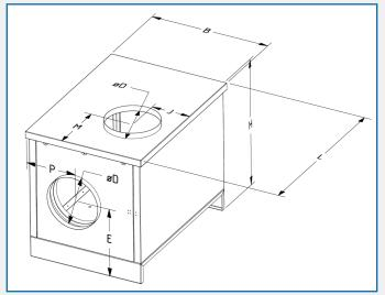
NOTE: When the fan is built into a soundbox it comes without feet. Custom versions such as AISI 316L are available on request at an additional charge.
