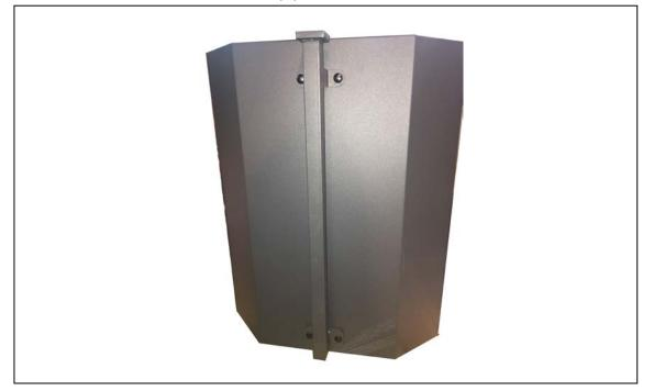
Step Forty Seven: Take the one of the cover plates, (2) 1/4"\*1/2" carriage bolts, (2) 1/4"\*OD19\*2t flat washers and (2) 1/4" hex nuts and secure the cover plate to the opening on the top of the drum. For the bottom holes do the same, but first use foam tape to cover the square opening before bolting on the cover plate.
