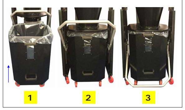
Step Forty One: Make sure when aligning the drum that both the left and right side lift plates are over the topping on the foot peddle bar assembly before lifting the foot peddle bar up. When not aligned, the drum will not be fully sealed and will interfere with the air flow.
