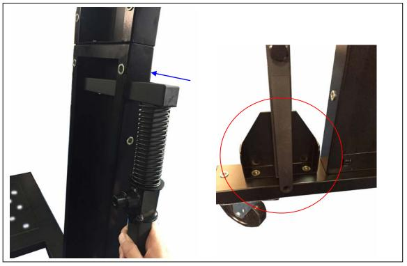
Step Seventeen: Secure the foot peddle support to the lower upright support panel using(4) 5/16"\*1/2" carriage bolts, (4) 5/16"\*OD18\*2t flat washers and (4) 5/16" hex nuts. Then secure the foot peddle bar to this support using (4) 5/16"\*1-3/4" hex bolts, (8)5/16"\*OD18\*2t flat washers and (4) 5/16" hex nuts. Follow the same steps for the opposite side.
