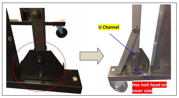
Step Nineteen: Attach the cover plate over the foot peddle assembly. Secure using (6) 1/4"\*3/4" hex bolts and (6) 1/4"\*OD19\*2t flat washers. Follow the same steps for the opposite side.
