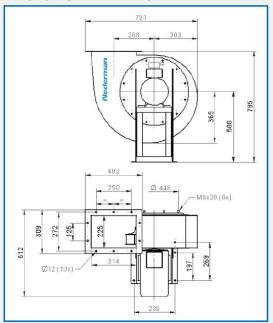
NCF 30/25 Duct inlet diameter 315 mm Duct outlet diameter 400 mm
